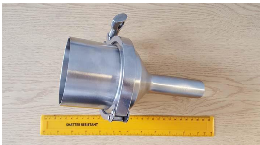
Figure 1. A filter leaf used for evaluating the filtration characteristics of a suspension.
