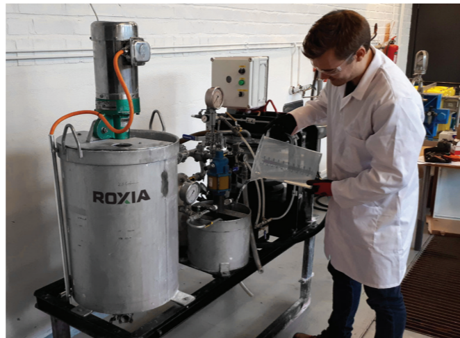
Tower press test unit simulates the operation of the full-scale industrial filter.
