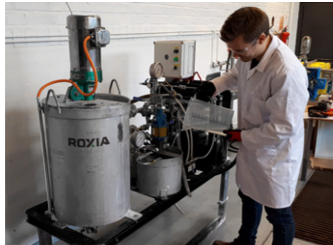
Tower press test unit simulates the operation of the full-size industrial filter.
